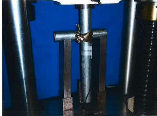
Photograph of Setup for Slipping Force
